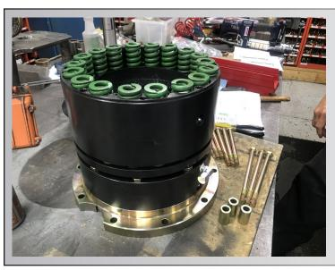
Slide the Chuck Housing 55-0006 into the Actuator Sleeve 55-0001.
