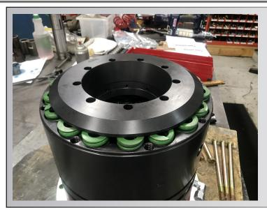
Insert Chuck Bowl 55-0005 into the Chuck Housing 55-0006. Align holes with the Bottom Spacers 55-0012
