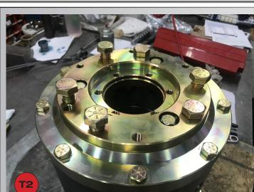
Install the Top Cap Adapter 55-0004 using the 6x 3/4-10 x 1-1/2" Grade 8 Yellow Zinc Finish Hex Cap Screw 15359. Torque bolts @ 110 ft-lbs.
