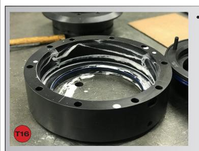
Lubricate the inside face of the cylinder with grease. We suggest White lithium grease as shown in Tool List.
