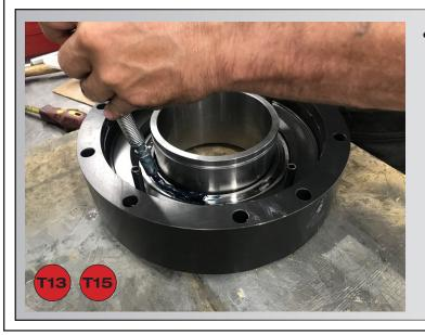
Install the largest of the 2 steel rings composing the **Thrust Bearing 15-51130** with the groove facing up and fill with grease.
