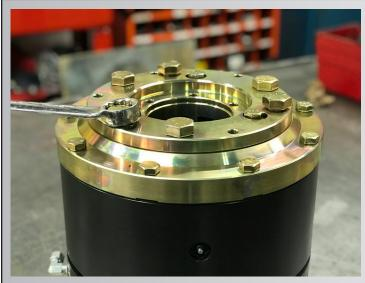
Remove the 6x 3/4-10 x 1-1/2" **Grade 8 Yellow Zinc Finish Hex** Cap Screw 15359 holding the Top Cap Adapter 55-0004.
