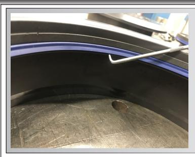
Install U Cup Seal Ø8-1/4"
