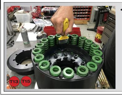
Put grease on the inside of the **Chuck Housing 55-0006**.
