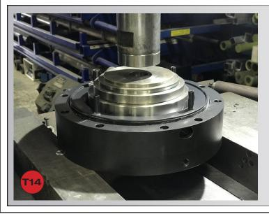
Push Chuck Piston 55-0010 into the Chuck Cylinder 55-0007 until it can go no further. The Chuck Piston 55-0010 will come out underneath the Chuck Cylinder 55-0007 9
