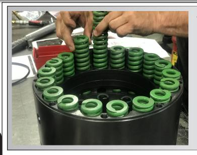
Insert the 21x Compression springs 55-0023 into the Chuck Housing 55-0006.
