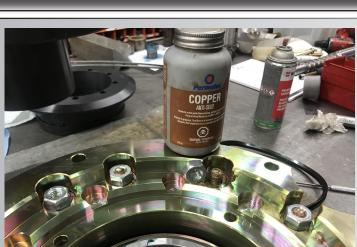
Install the Chuck Adapter 55-0008
