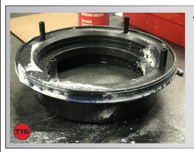
Lubricate the outside face of the **Chuck Piston 55-0010** with grease.
