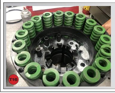
Insert 9x Bottom Spacers 55-0012 into the Chuck Housing 55-0006 until they are approximately halfway.
