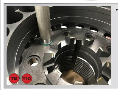
Press the 9x **Oil Seal 13-7415** into the pockets of **Chuck Housing 55-0006**. A special tool is recommended.
