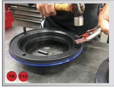
Install 4x 3/8" x 1-3/4" Plain Finish Steel Slotted Spring Pin 64313 into the Chuck Piston 55-0010.
