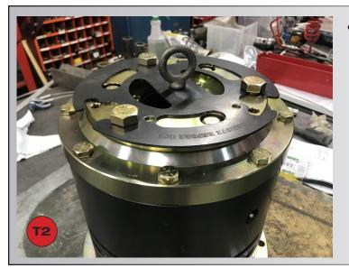
This step is optional, but a transport plate can used to help manipulation of the chuck. Remove before use
