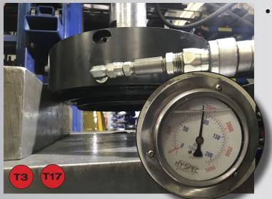
Install fitting 90° M-JIC #6 / M-NPT #4 2501-0604 and test the assembly for leaks. Leave the pressure ON in the hydraulic press and test the system around 1500 psi. Wait 15 minutes. If a leak occurs, it should show rapidly. If there is a leak, remove the pressure and disassemble the piston and Cylinder and check for seal damage. Also make sure seals were installed with the lips pointing in the right direction.
