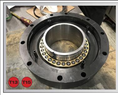
Insert the center brass ring of the Thrust Bearing 15-51130 and pack with grease.
