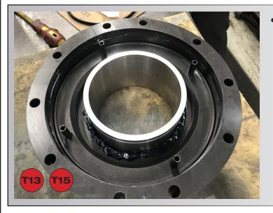
Fill the cavity with grease. We recommend using Castrol Pyroplex Blue grease or equivalent.
