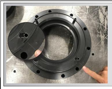
Insert the Chuck Piston 55-0010 into the Chuck Cylinder 55-0007 making sure the <u>spring pins are</u> <u>aligned</u> with the marks on the Cylinder
