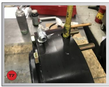
Install the 1/4-28 Straight Steel Zinc Self-Tapping Grease fitting 58834.
