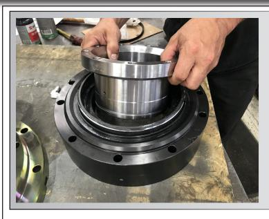
Insert Actuator Sleeve 55-0001 into the piston/cylinder assembly and turn over
