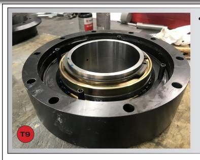
Insert **Retaining Ring 55-0014** into the actuator Sleeve groove. Use reataining ring pliers for this step.
